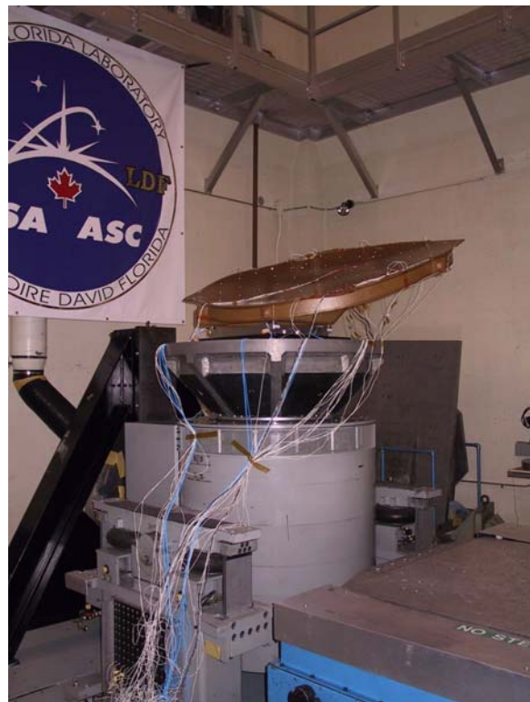
Figure 2: Z-Axis Driven Base Modal Test - Antenna
